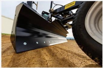
The Level Best Precision Blade Grader is designed for precision grading of flats, crowns and 3-D terrain
